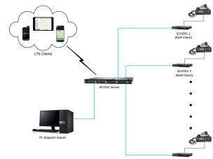
Note: LTE Clients may connect to the JPS PoC Server over either WiFi or a broadband connection. PC Dispatch clients may be wired, wireless, or over a broadband connection
